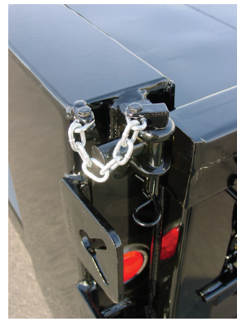
Double acting tailgate with drop pin upper hardware
