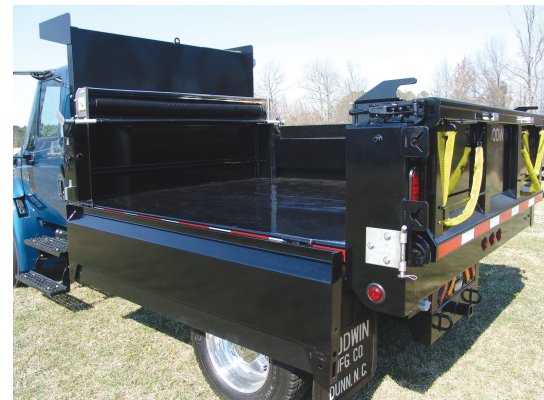
Optional drop sides in the down position. The side easily unlatches with a single handle and folds down lower than the body floor. Body shown with additional options.
